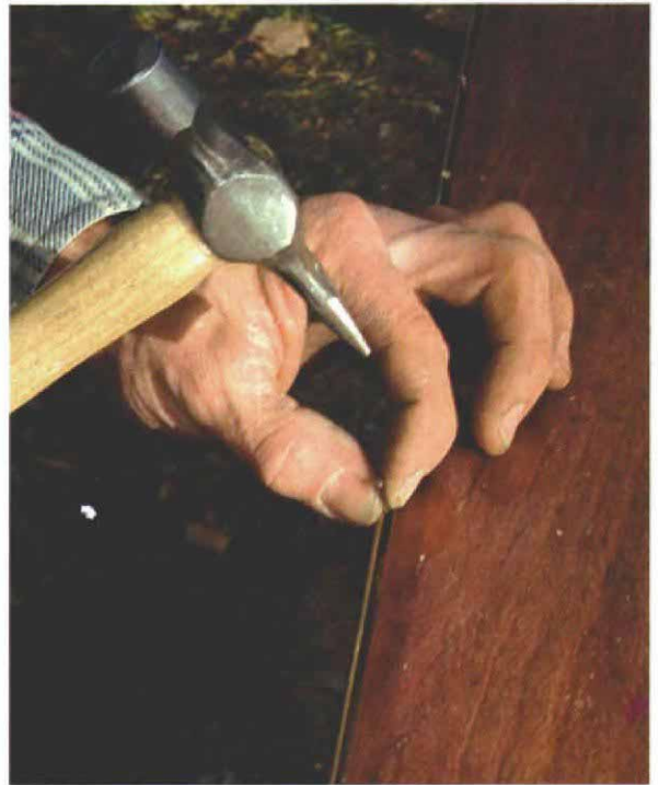
Brass nails hold the strips. A narrow-headed Warrington hammer starts small brass nails that are then driven home with a hammer and a nail set.
